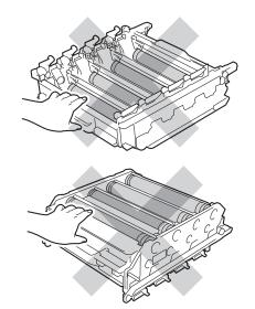
7 Turn the drum unit over by holding the green handles. Make sure that the drum unit gears (1) are on the left hand side.
